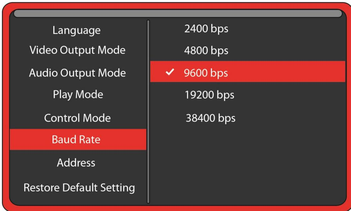
The baud rate is the speed of the serial communication and should match the settings on your external controller.
