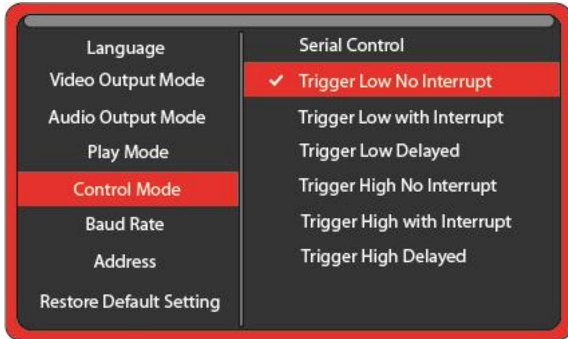
**Serial Control** is to use a Hydra® input expander or external show control device or micro controller like a PIC, Atmel, Arduino, Raspberry Pi, or etc. using serial communications.
