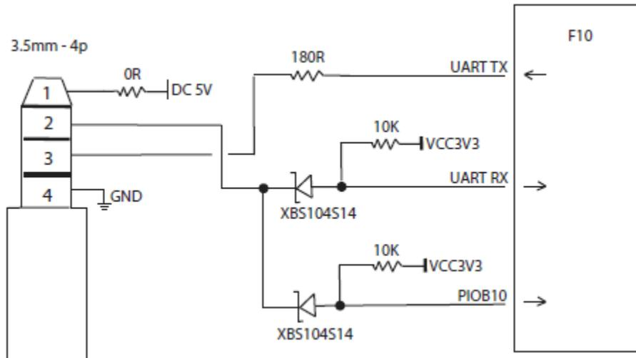
The Sprite is designed to work with 3 to 5 Volt TTL level serial data.
