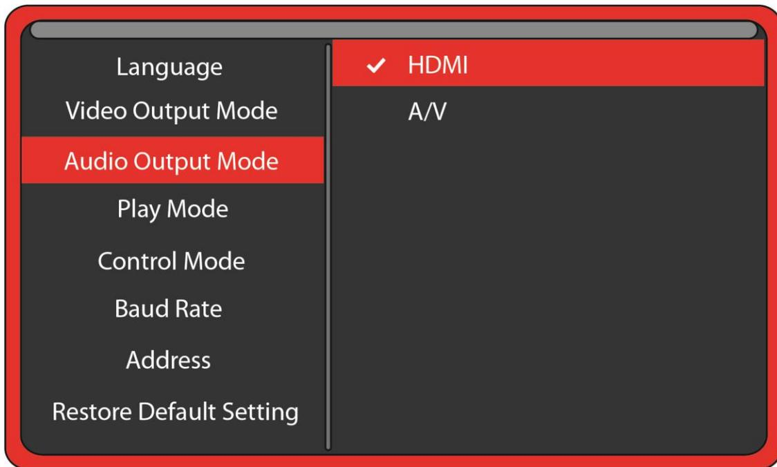
Select **HDMI** to route the audio only through the HDMI cable to your monitor or amplifier with HDMI input.
